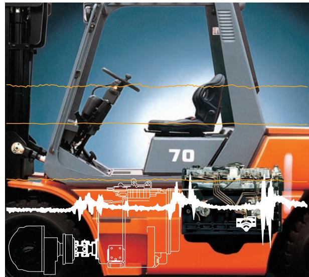
The 5-series uses a full-floating system that vastly reduces the amount of engine vibration transmitted to the frame, assuring a ride of unmatched comfort. This promises not only more comfort for the operator, but greater frame durability as well.
